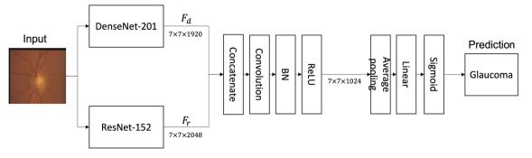
Figure 2. The architecture of the proposed GlaucomaNet.
